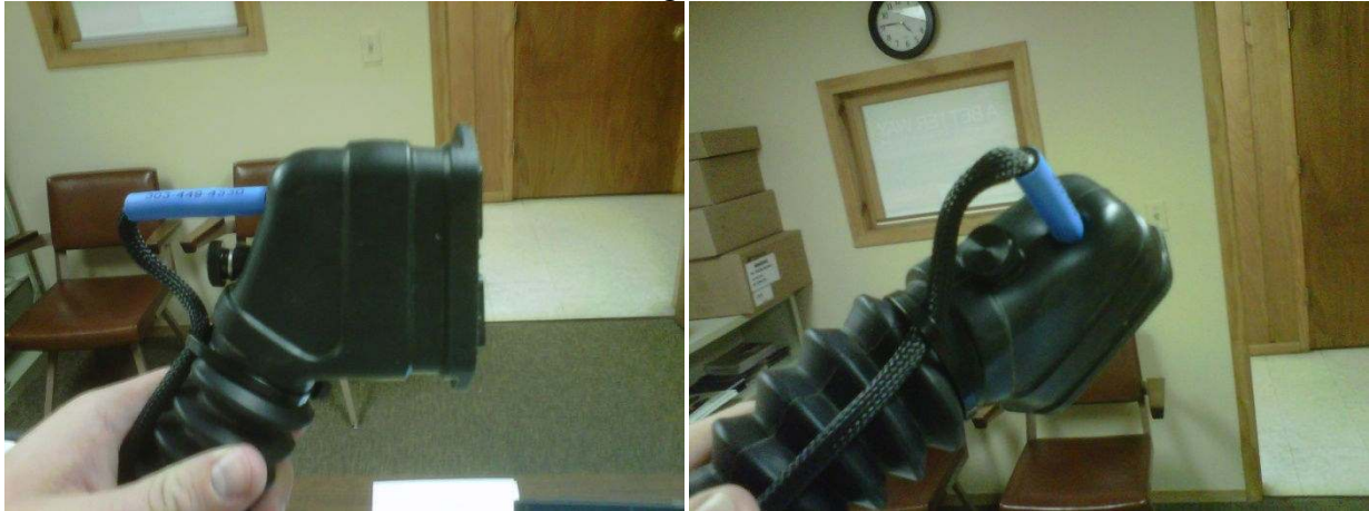
Example of how to connect the data power cable into the boot for the AGI-3 Data connector
