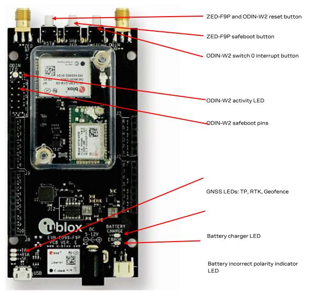
Figure 6: Switches and LEDs
