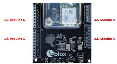
Figure 54: C099-F9P Arduino connectors
