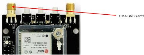
SMA GNSS antenna connector
