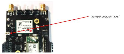
Figure 19: C099-F9P rover jumper position
