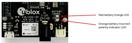
Figure 11: Battery charge status LED
