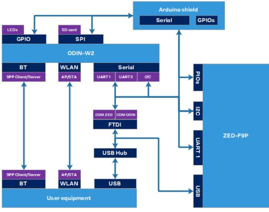
Figure 4: C099-F9P block diagram
