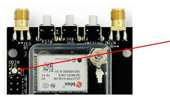
Figure 8: ODIN-W2 Activity LED position on C099-F9P board
