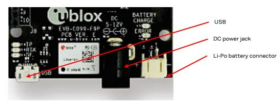
Figure 9: Power connections
