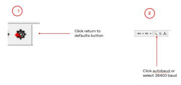
Figure 36: Return receiver to defaults and select 38400 baud
