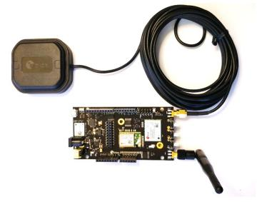
Figure 1: C099-F9P board and antennas
