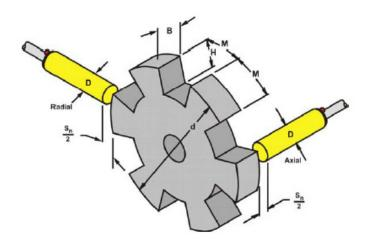
greater than or equal to the diameter of an embeddable proximity sensor.
