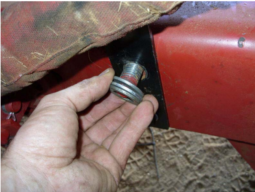
Figure 3-22 Placing Washers on Wheel Angle Sensor Bracket
