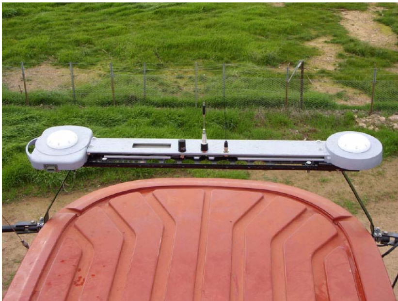
Figure 5-7 Roof Module Installed
