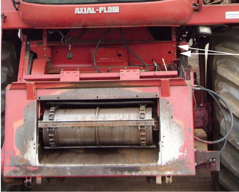
Figure 2-12 Mounting Bolt Location
