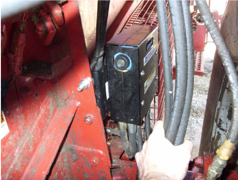
Figure 2-19 Valve Mounted (shown with hoses connected)
