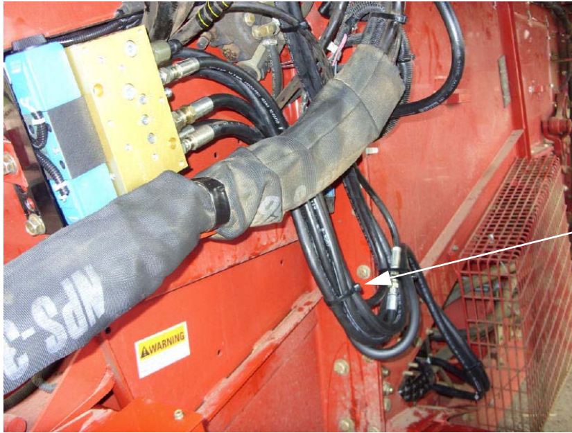
Figure 2-29 Hose Routing Example
