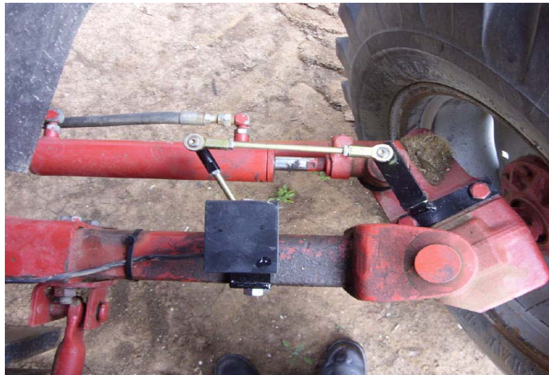
Figure 3-14 Full Right Wheel Angle Sensor Test
