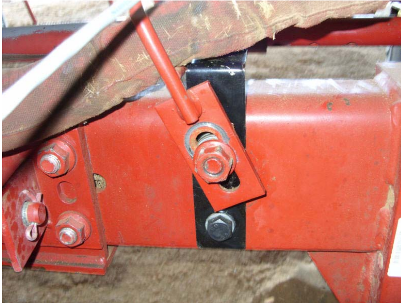
Figure 3-23 Hose Bracket Reinstalled
