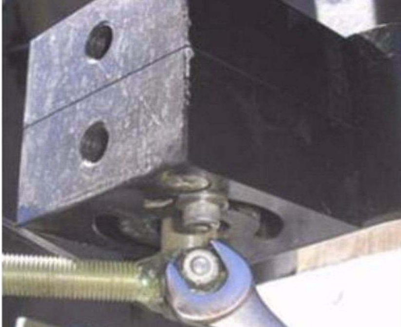
Figure 3-33 Tightening Wheel Angle Sensor Linkage Rod Connection
