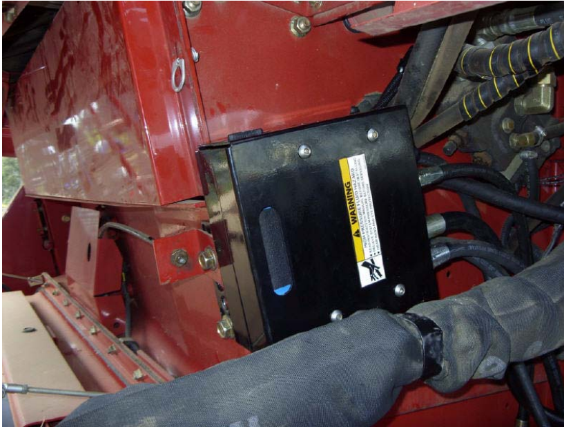
Figure 2-15 Steering Valve Mounted (shown with hoses connected)
